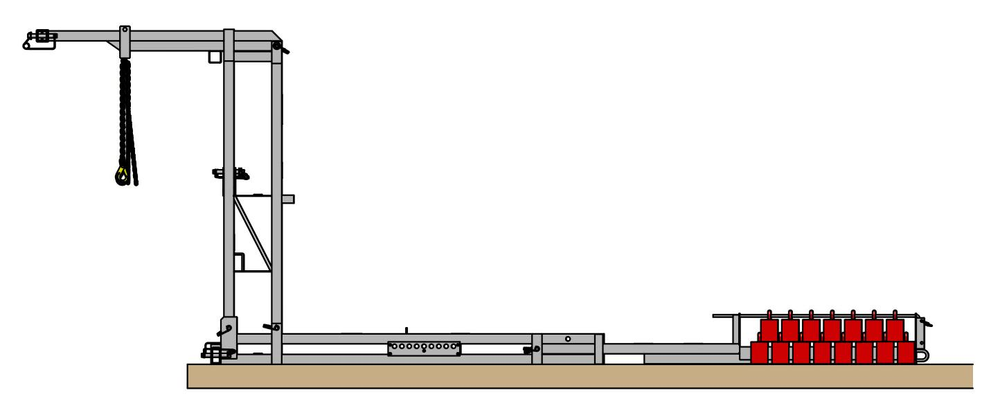
Step 1. Assemble the Suspension Frame per the instructions in the Chute Hoist Installation Manual
