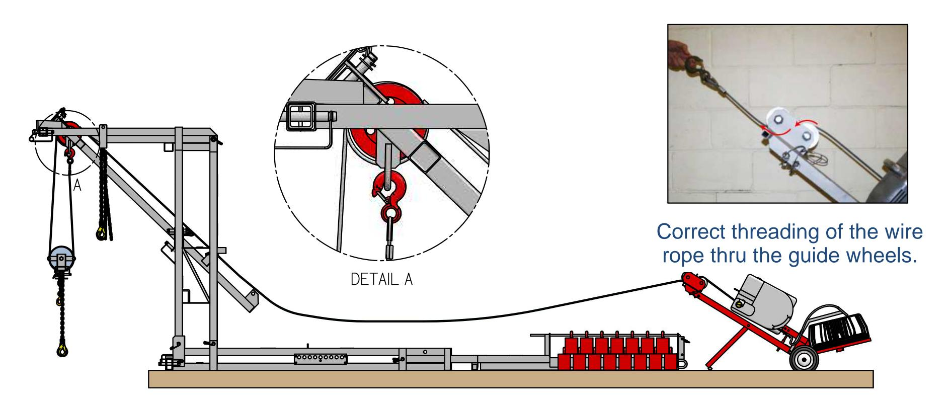
Step 2. Install the Fishpole on the frame as shown above
