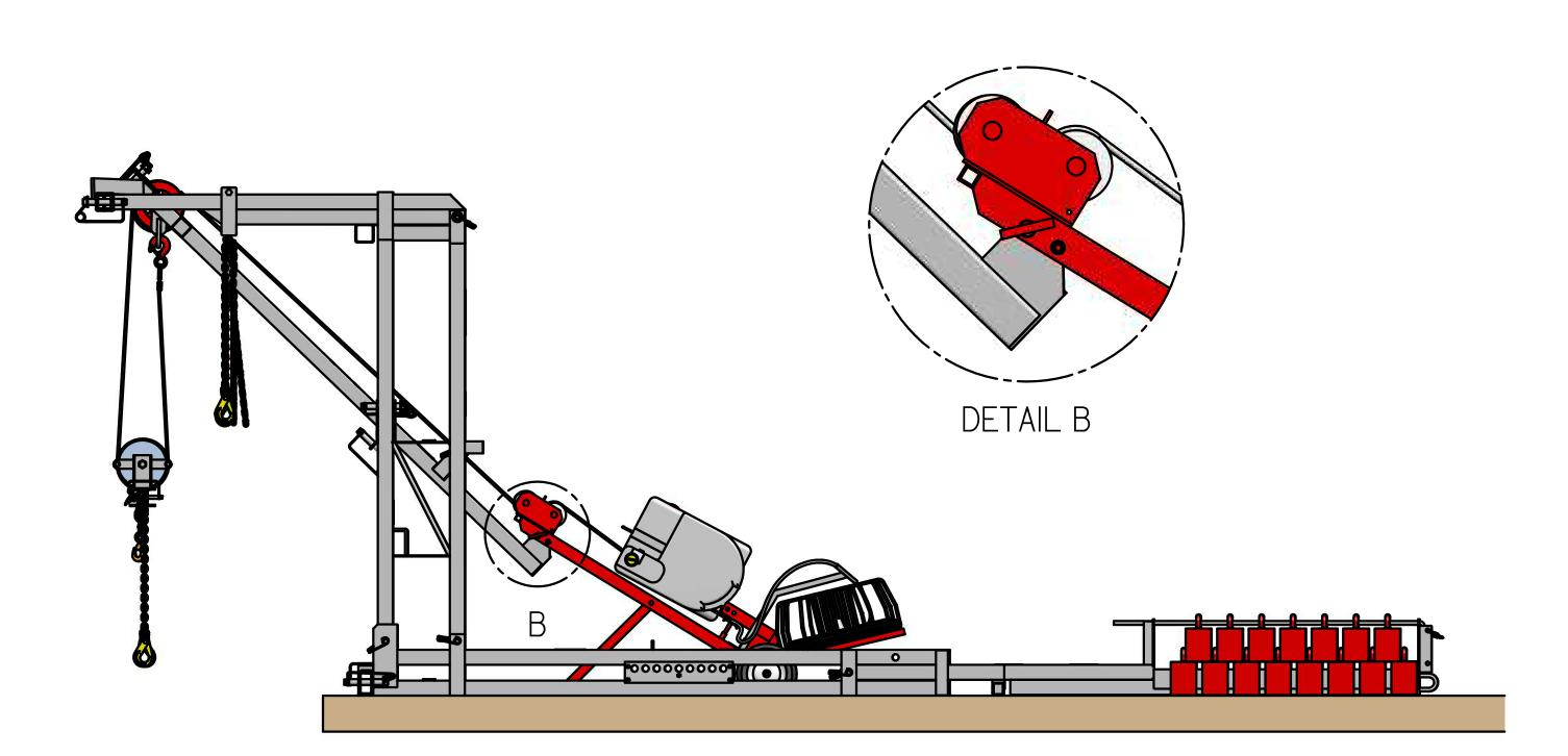
Step 3. Roll the EFA into position and pin the EFA to the butt of the Fishpole. Use the larger of the 2 pins. The large pin matches the pin diameter found on the Tractel **T516** manual winch box (the small pin matches the pin diameter of the Tractel **T508** manual winch box).
