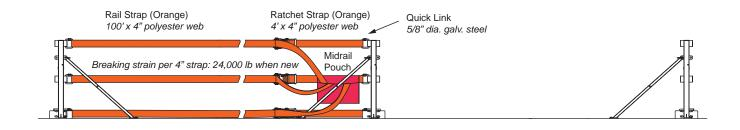
STEP 3: Tension the rail straps. Install Anti-Deflection Posts every 10 feet. Install optional Padlocks (P). For falling object protection attach StrapRail® Netting to the barrier.
