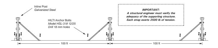
STEP 2: Use Quick Links to connect the Rail & Ratchet Straps to the Inline Posts.
