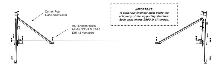
STEP 2: Use Quick Links to connect the Rail & Ratchet Straps to the Corner Posts.
