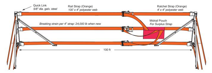
STEP 3: Tension the rail straps. Install Anti-Deflection Posts every 10 feet. Install optional Padlocks (P). For falling object protection attach StrapRail® Netting to the barrier.
