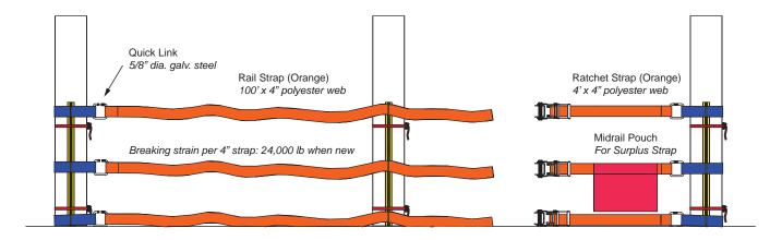
STEP 3: Tension the rail straps. Install Anti-Deflection Posts every 10 feet. Install optional Padlocks (P). For falling object protection attach StrapRail® Netting to the barrier.
