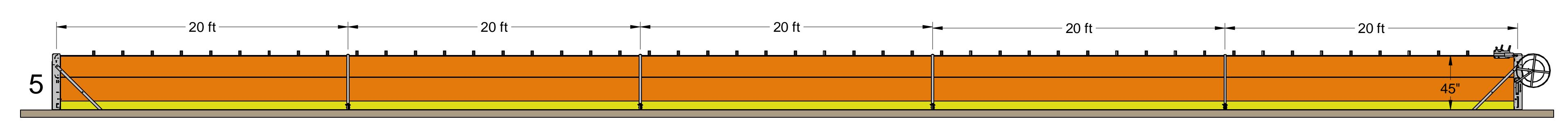
Pin the intermediate posts to the wire on 20 ft spacing. Bolt the posts to the slab. Use 2 anchor bolts per post (HILTI HUS KH-EZ 5/8" x 5.5"). The installed RopeRail™ system is under continuous load test and meets OSHA 1926.502.
